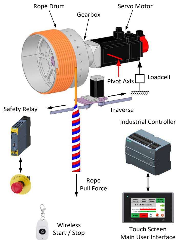
Bell motion is modelled in software by solving the equations of motion of both bell and striking clapper within a small industrial controller to provide an instantaneous angular position in real time.
