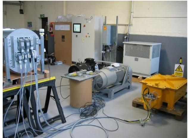
This was an 18-month R + D project to design and build the power conversion and control system for a prototype semi-submersible tidal generator. I was responsible for all electrical engineering and control activities which included: -
